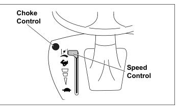
Figure 10. Independent Speed and Choke Controls
